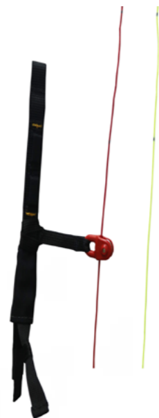
Step 8. Pass the main line inside the pulley
