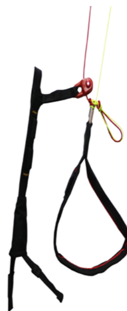
Step 1. Open the toggle knot.
